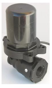
Type: **Compact actuated ball valve** (type 2008) Material: **GRPP** (Glass reinforced Polypropylene) DN: **15-20** Actuator: **SM1** Actuator waterproof (IP65), Options: **available in 2 or 3 ways** Weight: **1,2kg** Remark: actuator with quick release cover (bayonet fitting)
