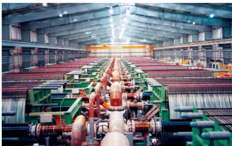
Pressure is 0 bar in the electrolyser and temperature is 90°C. Everything that comes out of the electrolyser is at this same pressure and temperature.
