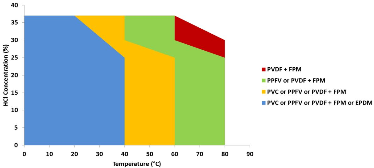
HCL also returns to the plant for the iron exchange bed regeneration and brine acidification. GRPP/EPDM/FKM ball valves can be used for this.
